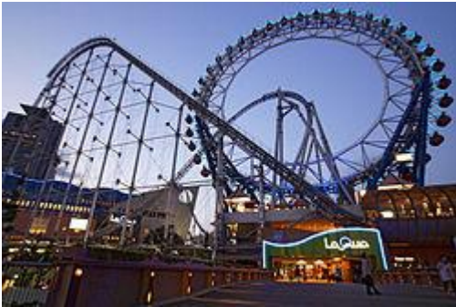
The Big O at Tokyo Dome City is a hubless Ferris wheel .
