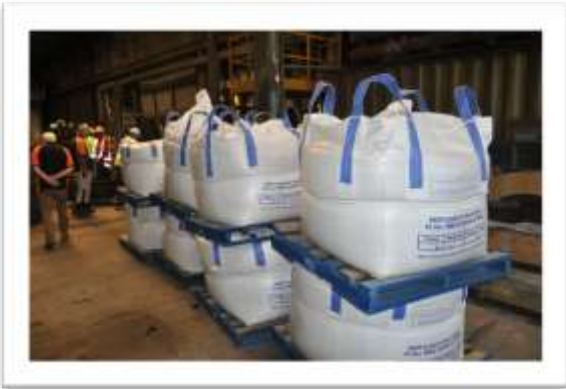
Silica sand the medium which is placed around the patterns to produce the casting .
