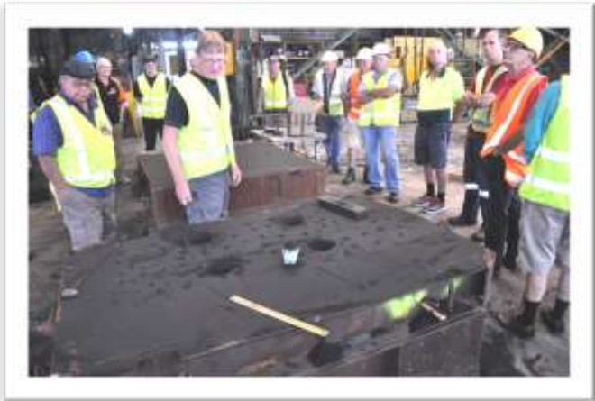
The sand box complete and ready to be poured
