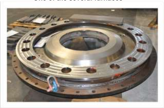
Machining a housing after casting and heat treatment
