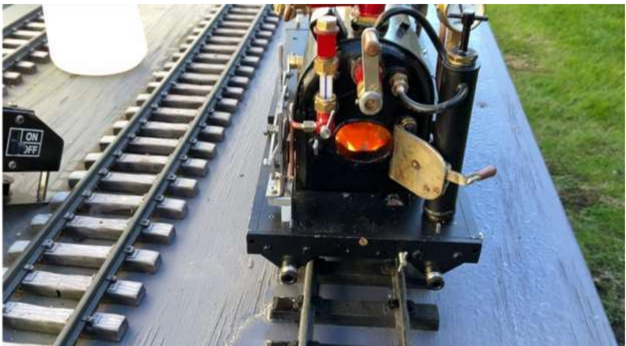
This shows the coal burning nicely and working with the steam blower.
