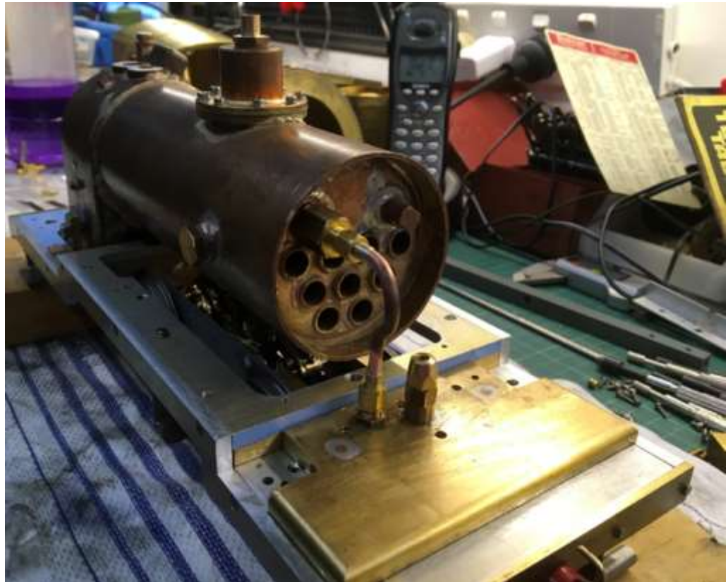
The steam feed pipe in place and the boiler mounted.
