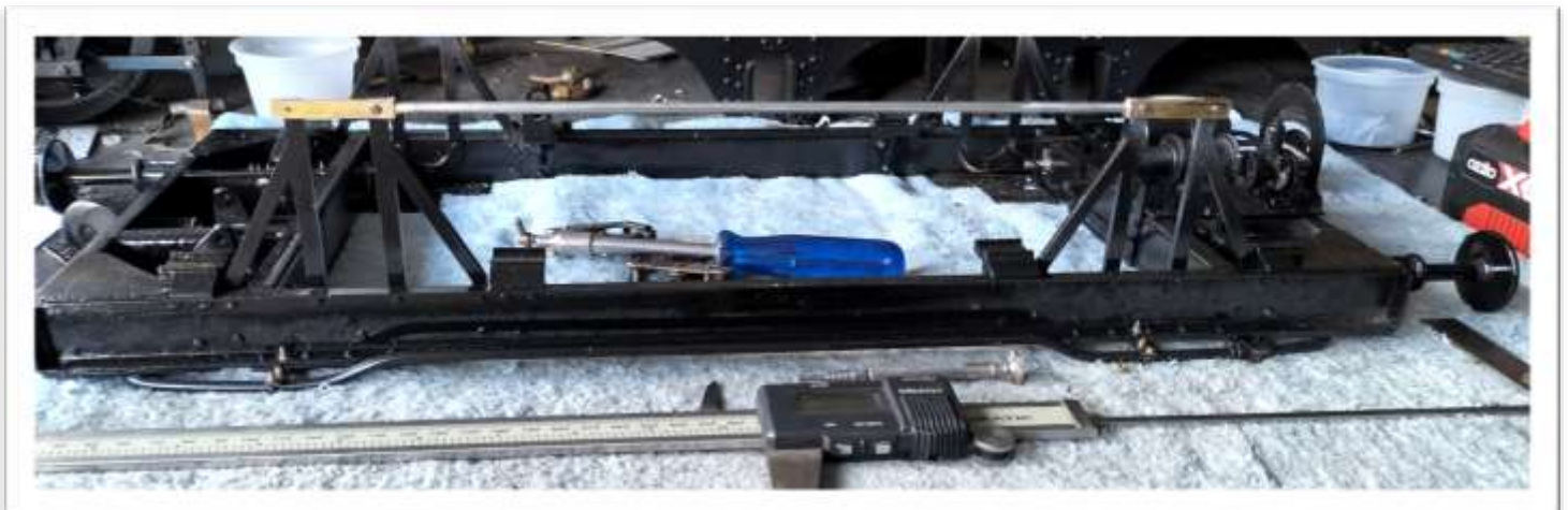
Trial fitting of braces to check length.
