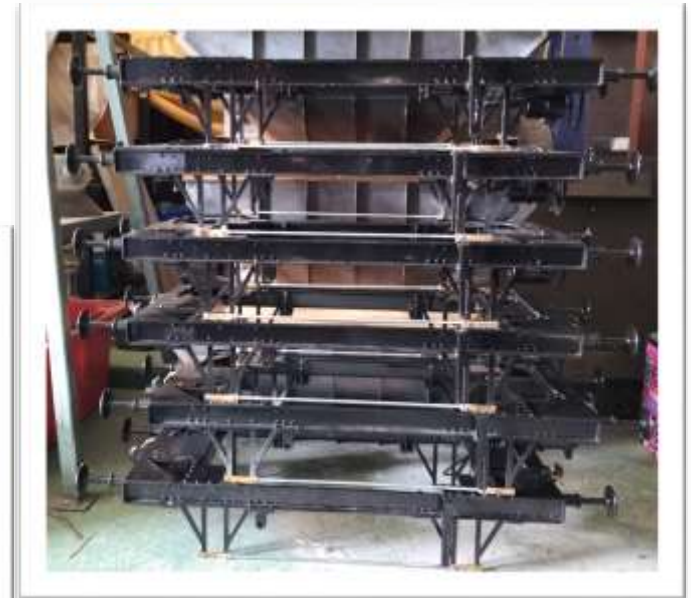
Top : Jig to hold everything in place for silver soldering.
