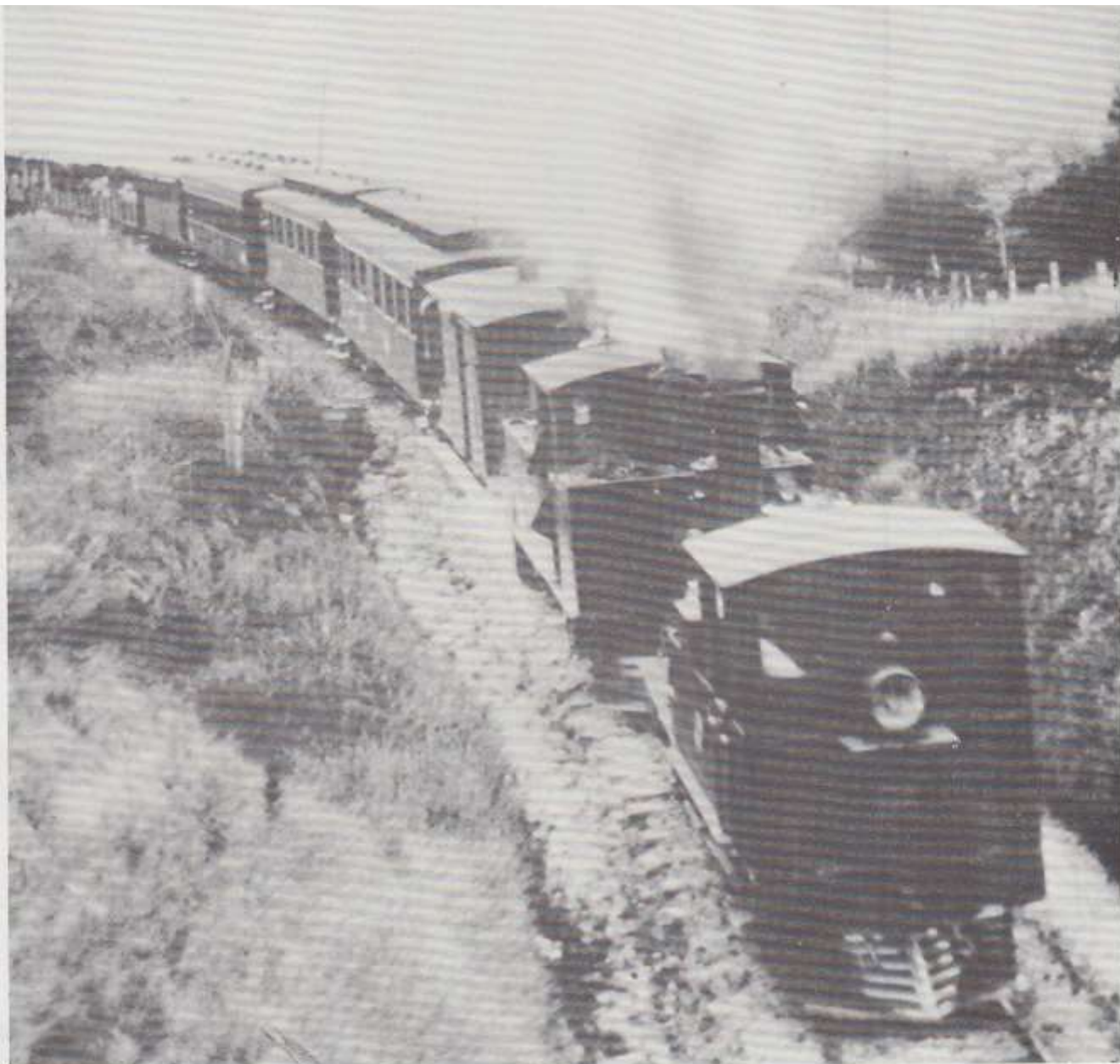
Ascending from Annesbrook Crossing to Bishopdale, about 600 yards from the crest of the 1 in 35 grade. The locomotives are D 144 and Fa 373 with a coupling bar between them. Then follows a four-wheeled guard's van, three bogie passenger cars, a six-wheeled C class car and a string of canopied high-side L wagons pressed into service as passenger conveyances. The train was returning from the Agricultural and Pastoral Show at Richmond about 1910. Photograph author's collection.
