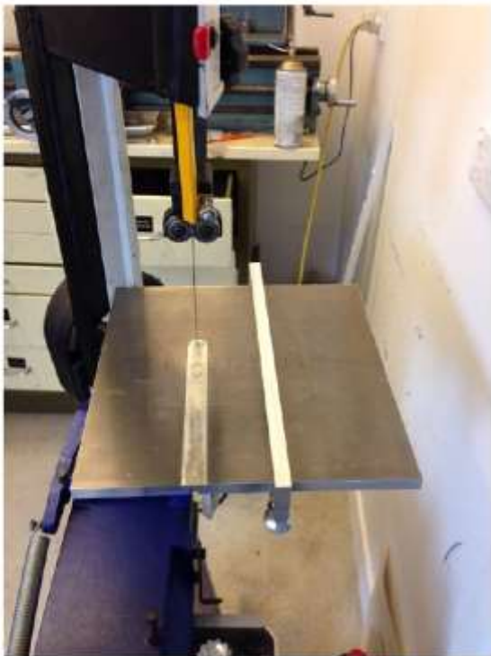
Photo 8 shows the finished table attached to the saw, with a fence. This was added to use for parallel cuts.
