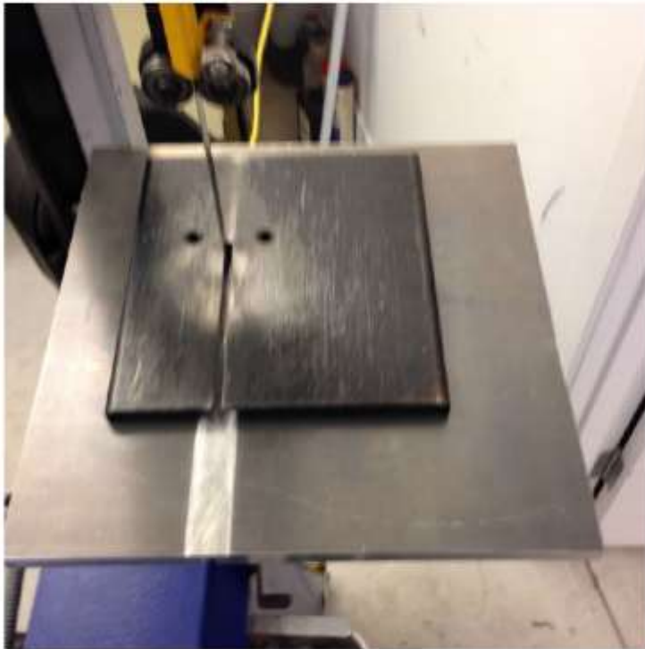
Photo 6 On the back is an other piece of plate with a recess cut in it that slips over the blade table.
