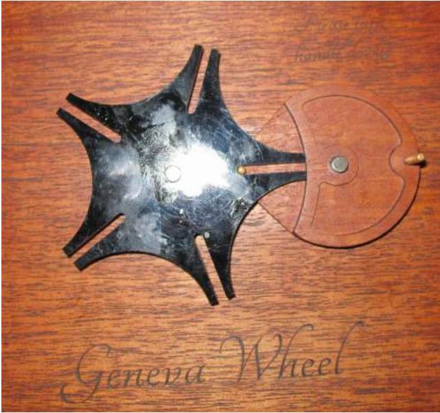
Murray de Lues showed some fine art on a paint brush. Also a Geneva Wheel, a device for indexing with locking rotational movement.,
