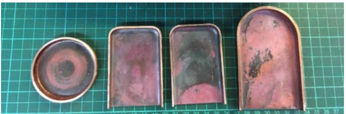
Boiler plates formed and ready for drilling.
