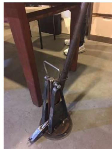
Russell Prout's tools for rerailling carriages and locos.
