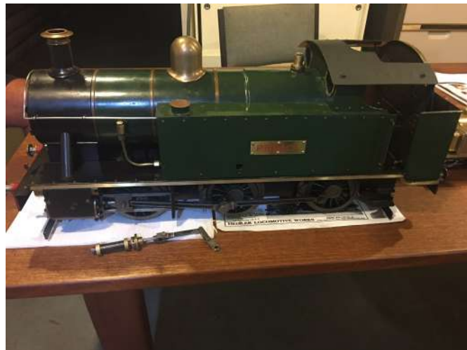
Ashleigh Grant's loco with Baker valve gear showing the actual valve mechanism.
