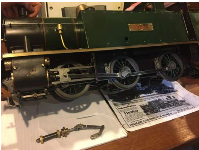
Ashleigh Grant's loco with Baker valve gear showing the actual valve mechanism.
