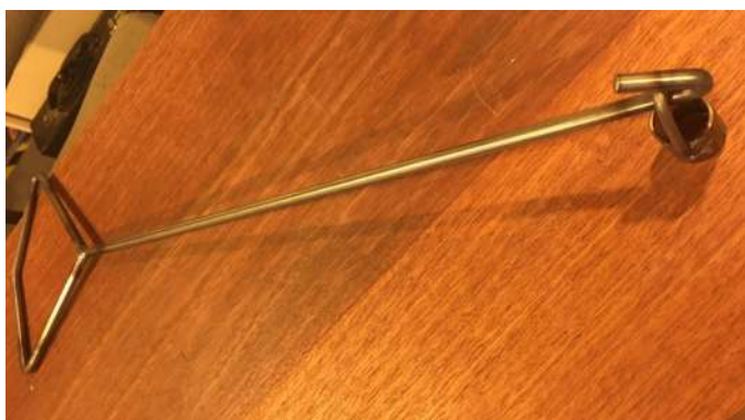
Russell Prout's tools for rerailling carriages and locos.
