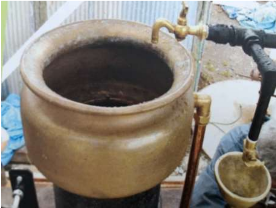
Fig 6 shows some of the many parts for which patterns were made and pieces cast on site.
