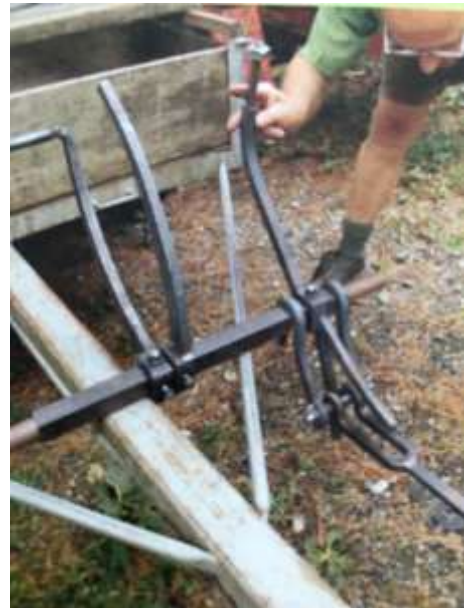
Fig 4 Shows some of the many hand forged details that made up the links, arms and operating apparatus that enables the machine to self start and run without manual intervention.
