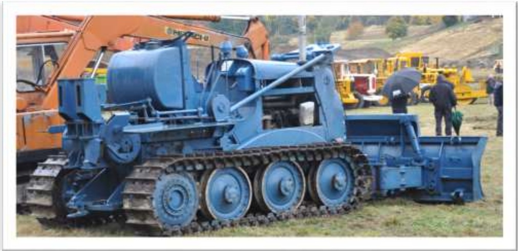
An English, Vickers Vigor dozer, track gear design based on the military tank engineering, powered by a Rolls Royce C6 diesel. (1951—1958)
