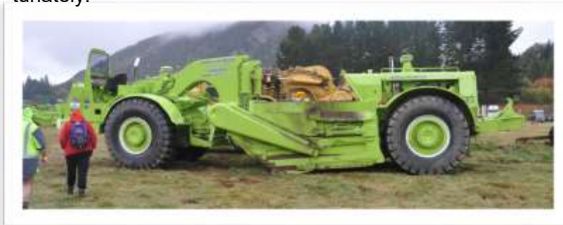
Terex TS18 scraper, 18cubic yards capicity 21 cy heaped, powered by 2 X 6/71 GM two stroke diesels.
