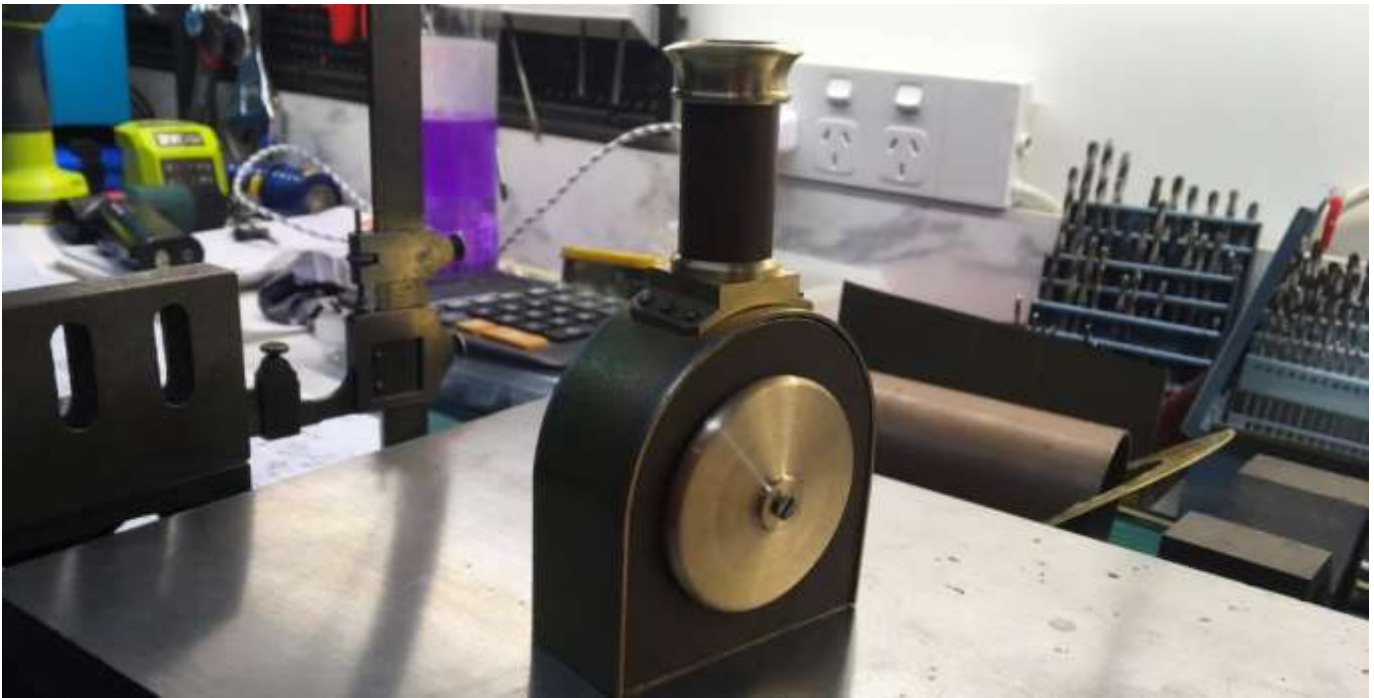
Smoke box with door temporarily attached
