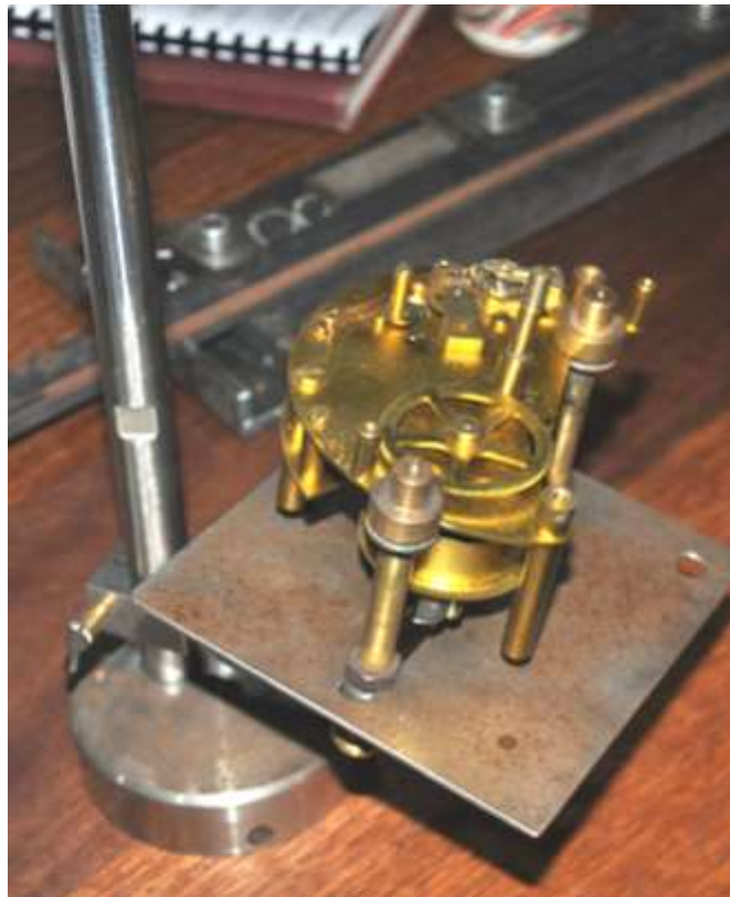
Jig to hold clock mechanism whilst under repair, Roy R.
