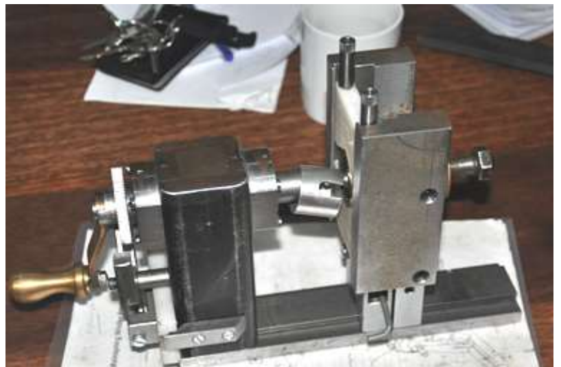
Tool to allow releasing the energy of clock springs. Roy R
