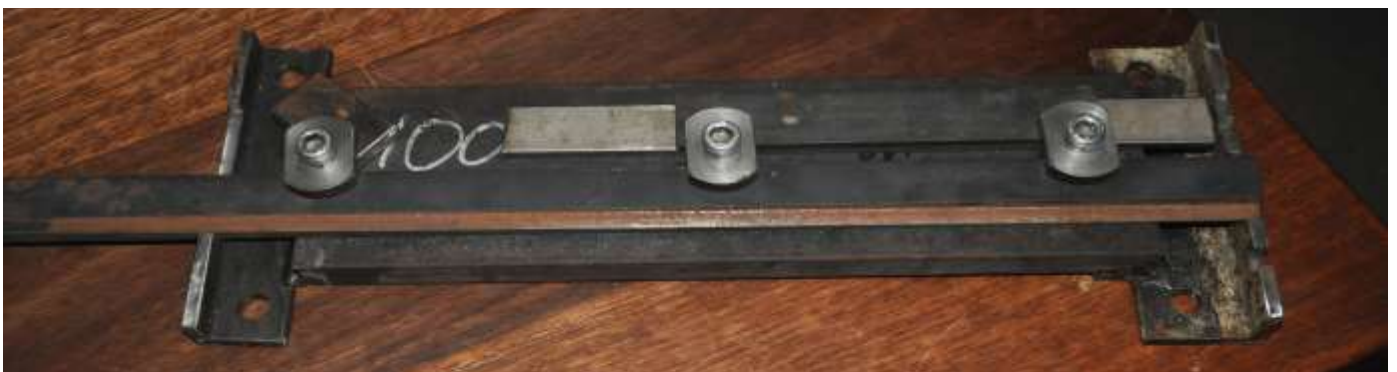
Russell P has built this jig to machine track rail for machining lead into points.
