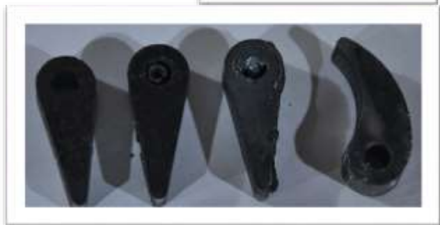
Ross had some parts laser cut for the forward/reverse mechanism on his traction engine.
