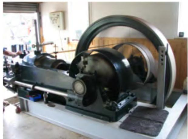
Actual details are not known but would have been in the vicinity of 30 – 40 hp and ran on producer gas from an onsite retort. It has a flywheel of about 6 feet and bore of 10 inches (best guess). When installed the engine refused to run on the producer gas. It was believed that at the altitude of 2500ft was too high to be able to run, and the project was abandoned despite there being a reasonable amount of ore ready to be crushed.
