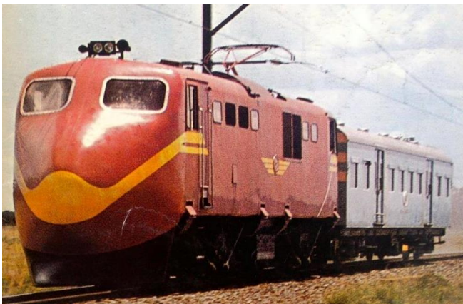
World record holder on narrow gauge, set in October 1978. Speed 245 kph. SAR Class 6E1 loco with modified DC pantograph and Scheffel bogie.
