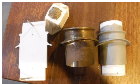
Printed chimney mould
