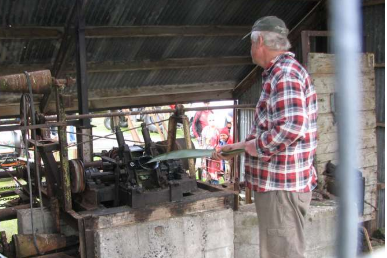
Operator feeding the stripping mill, note only single leaf.
