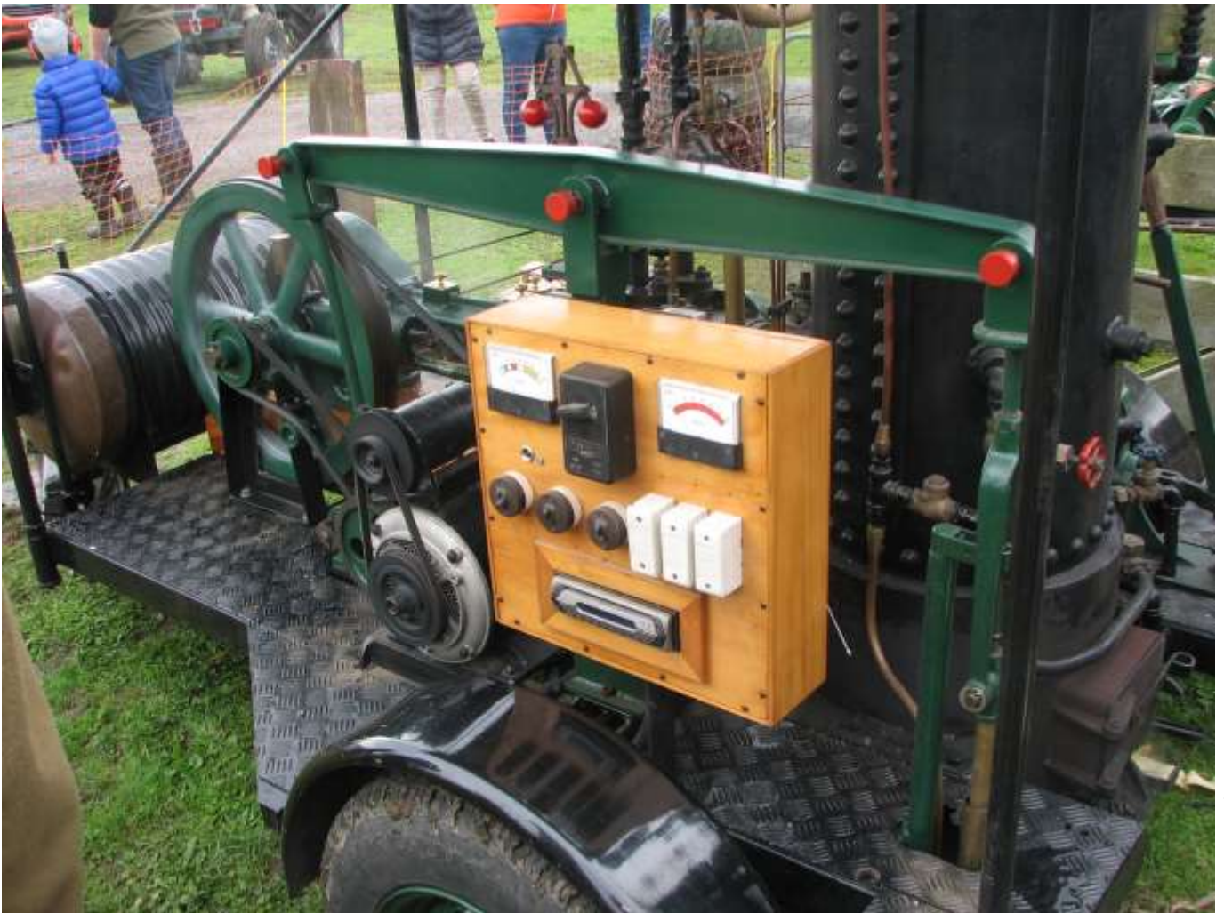
The boiler (right) and the continuous running engine with generators, water pump, holding tank all on a trailer.
