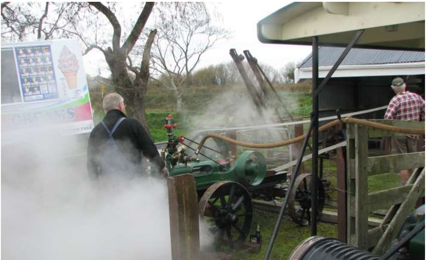
The Stripping Mill engine. Note the long flat belt drive .
